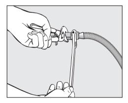
Using two adjustable wrenches tighten all connections.
